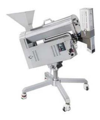
HSLC100 Capsule Polisher & Sorter is a polishing and sorting machine for capsules. It can not only be used to polish capsules and eliminate static electricity on capsules, but also automatically remove unqualified capsules with defects such as low weight, empty shells, fragments and capbody separation.
