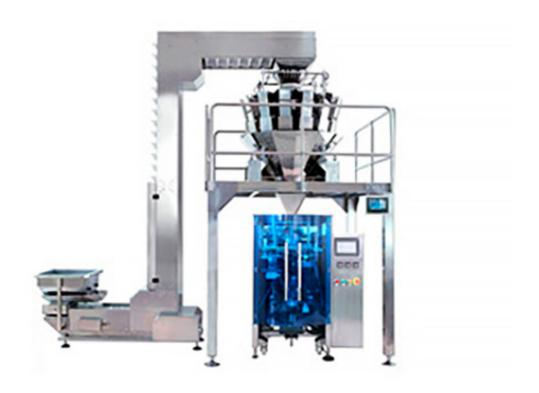
The automatic packaging machinery to complete the bag, measuring, filling, nitrogen, play yards, cut bags and so on.
