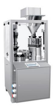
It adopts intermittent motion and multi-position tamped dosing method to complete capsule orientation, separation, filling, closing and ejection etc. With different size parts the machine is suitable for size 00 to size 5 of empty capsules.
