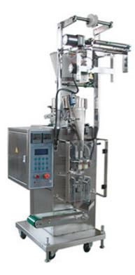
DXDK 80C automatic sachet packaging machine can do granule material packing in the small sachet.
