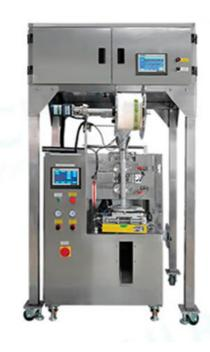
SJB01-06 is a triangular bag filter bag tea bag machine that can be configured with 1-6 weighing devices according to your needs.
