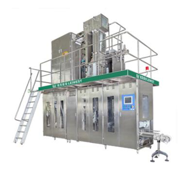
LWG6CF flexible aseptic filling machine adopt flexible design, quick change package type, 30 minutes can replace the same section of different capacity package type. One working day can replace the different section of different capacity package type.
