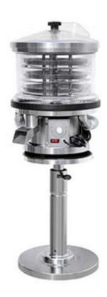
CFQ300 Tablet Deduster is suitable for dust removal of various shapes of tablet. The production process is intuitive and visual. Adding powder isolation device between each layer of sieving plate effectively separates tablets and dust. The parts in contact with tablets are made of SUS316L / SUS304 stainless steel. This machine can be equipped with any tablet press machines as an ancillary machine.
