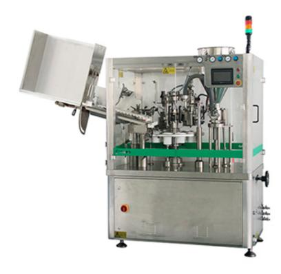
The Machine can be used in the industries of pharmaceutics, foodstuffs, cosmetics, daily chemicals for smoothly and accurately filling all kinds of pasty and viscous fluid and the materials alike, into soft metal tubes and then carrying out tube end folding, sealing and lot number embossing.
