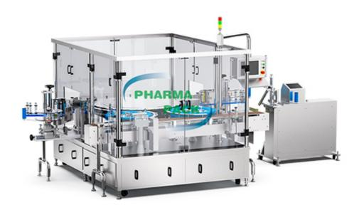
With the experience in vial labeling machine research and development, PHARMAPACK creates LFLB-1160R rotary round bottle labeling system, which is perfect with high speed and precision for different kinds of vials, such as ampoule, antibiotic, and oral syrup. It can be used offline or to be integrated with Coding System, Amouple/Vial Tray Packing System, Particle Inspection Machine and Cartoner.
