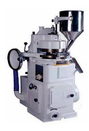
This machine is basic equipment that is suitable for continuously pressing the various granular raw materials into tablets. It is applicable in electronic, food, chemical engineering, commodity, pharmacy, etc. It also can press the blocky products of geometric shapes (round or annular), such as instance electronic element, camphor ball, accelerant and powder metallurgy products, etc.
