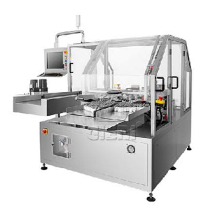
Applied to high precision labeling on penicillin vials, oral liquid, ampoules, Schering bottles, and other small pharmaceutical bottles, cosmetic bottles that can't stand very stably.
