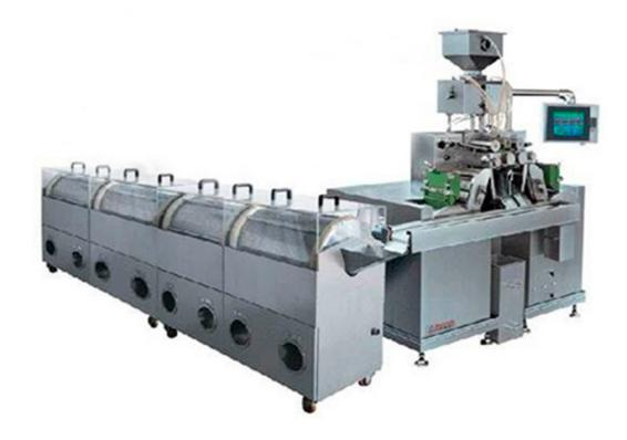
Model RG2-110 soft-capsule production line is a new generation of rolling-mold water-cooled soft-capsule line optimally designed and finely manufactured on the basis of foreign latest technology.
