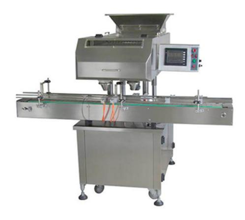
This high-speed tablet and capsule counter combines 16-channel counting heads over a dual-track conveyor on a single frame to double the throughput without doubling the floor space, achieving speeds up to 60 cpm based on 100-count bottles. The machine handles a wide variety of tablets, caplets and both hard and soft capsules of different shapes, sizes and properties.
