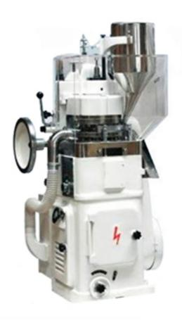
It is a new generation product by our factory, and this machine is a single roller continuous automatic tablet press for pressing various kinds of different shape tablets and plain tablets. It is mainly used in pharmaceutical industry and also the chemical, food, electronic industries.
