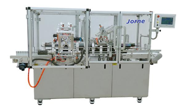
Vertical Cartoning Machine ZV40 is a mechanically driven, intermittent motion vertical cartoner, it is suitable for packaging cosmetic and pharmaceutical products that require vertically loading into a carton at speeds of up to 40 cartons per minute.
