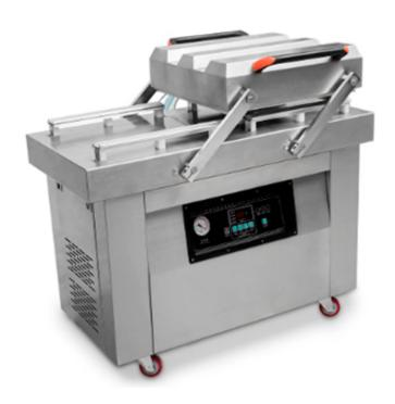
DZ-2SA series double chamber vacuum packing machine is featured by automatic processing of vacuumize, sealing, printing, cooling, which is used in vacuum packaging for food, pharmaceutical, aquatic, chemical and electronic industries. It can prevent the products from oxidization and mildew, as well as corrosion and moisture, keeping the quality and freshness of the product over a prolonged storage time.
