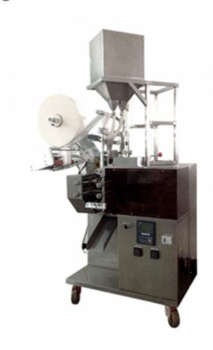
It is suitable for packing products with granule or powder shape.
