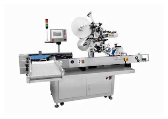
Horizontal feeding  $\rightarrow$  spiral separation of bottles  $\rightarrow$  batch number printing  $\rightarrow$  horizontal labeling  $\rightarrow$  online testing and exclusion  $\rightarrow$  finished product.
