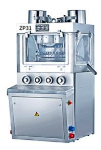
This machine is a double-press type continuous automatic tablet press machine for pressing granular raw materials into tablets. It is mainly used in pharmaceutical, chemistry, foodstuff, electronic industries and suitable for make large size tablets.
