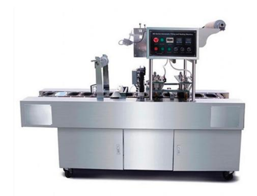
BG32A-1automatic cup filling and sealing machine is widely used in filling and sealing various kinds of plastic cups for liquid. It can automatically complete the processes of cup-dropping, filling, sealing, film cutting, code printing, sterilizing in ultraviolet radiation and cup-falling in one operation.
