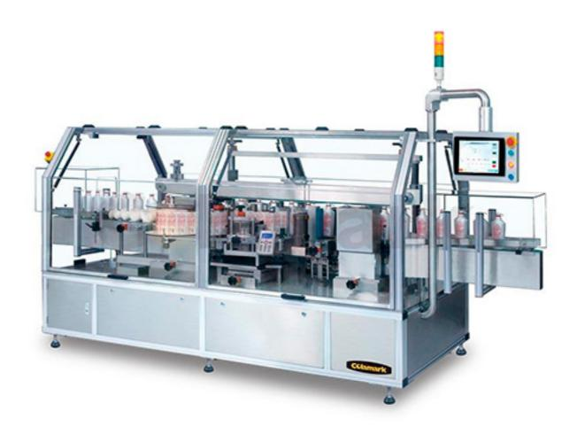
For front and back labeling on oval, rectangular, or other irregular shaped bottles in the cosmetic, daily chemical, food and beverage, and pharmaceutical industries. A920T offers high labeling precision up to ±0.5mm, and high speed up to 200 bpm.
