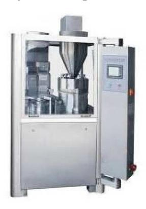
SPR-6 Automatic Capsule Filling Machine. Small volume, low consumption of energy, simplification in changing modules. Easy operating and cleaning. Adopt eliminating Ma's trough roller to transmit, less vibration, its noise is lower than 75dB while running at top speed. Dose difference is controlled within ±3%. The rate of capsule fling is >99%.
