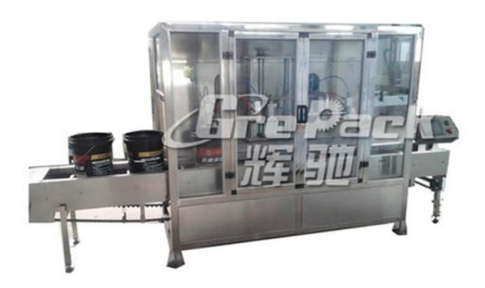
The weighing liquid filling machine adopts Mettler Toledo weighing module, combined with automatic filling technology, so as to realize high-precision dynamic metering and filling of liquid materials, and its metering accuracy is not affected by factors such as pressure, temperature, and air bubbles;
