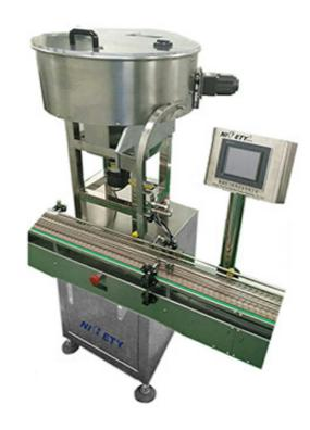
Used for automatically sorting, counting and filling canister dryers into bottles.
