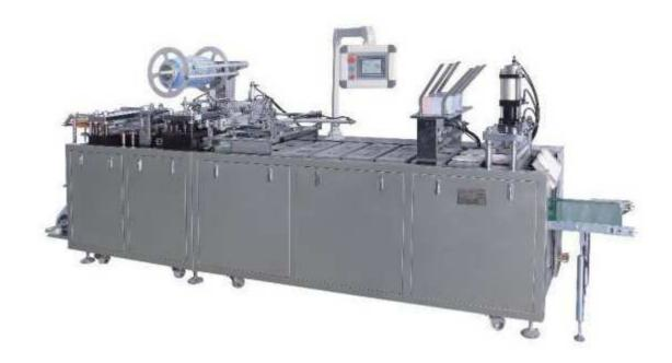
JP-500D automatic blister packing machine adopts frequency control of motor speed. Collecting machine, electricity, photo, air to integrate, and innovative design, Manufacture according to national standard strictly, flexible stroke, modularize station structure, easy operation, high output, low noise, and equipped with Beautiful out looking, this is the ideal packing machine.
