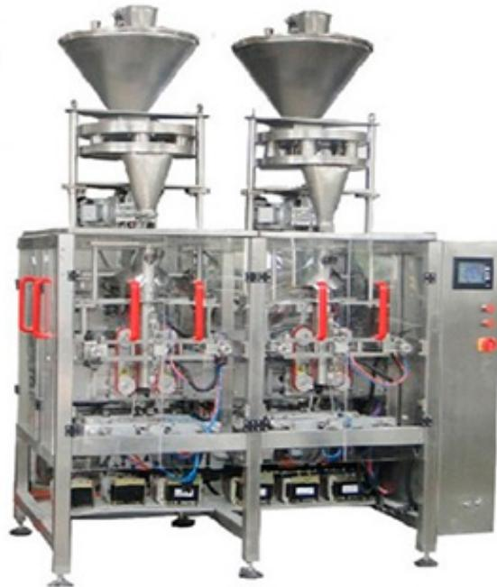
This packing unit consists of two vertical packing machine for bagging two sets cup filler for weighing, two screw elevator for feeding, two conveyor for taking off the finished bags. It integrates functions of automatic bag-making, weighing, filling, sealing, printing, punching, cutting and sealing into one. The advanced design has guaranteed this machine suits for different kinds of granules, like salt, rice, etc. Its adjustment, operation and maintenance are very convenient.
