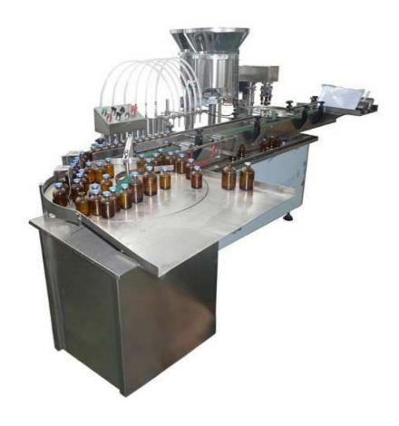
This machine is the main filling equipment of the bottle production line, which is mainly applied in the filling, plugging, covering and capping of 10-500 ml bottles. This machine combines filling and sealing, advanced design, compact structure, the Replacement of the bottles is very convenient.
