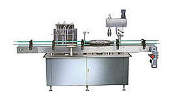
The linear filling capping machine named SD-ZGF-1000 linear filler capper is composed of bottle-setting, filling lid-laying and lid-rolling equipment. It is a kind of straight-line filling and lid-rolling machine for packing cosmetic liquids and creams both in plastic bottles and glass bottles.
