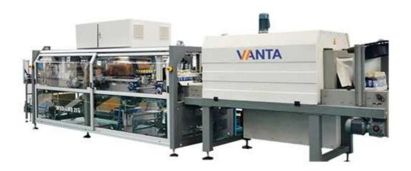
Automatic shrink wrapping machine packages bottles, cans, jars into film through continuous linear operation. The machine adapts to medium and high production line with its good stability and easy operation.
