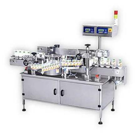
Fully Automatic, User Friendly, Sticker (Self-Adhesive) Labeling Machine Model OBSL-120D, Suitable to apply accurate Labels on Double Side (Front & Back) of Flat/Oval/Square shaped products having PET, Plastic, HDPE, LDPE, Glass or any other surface.
