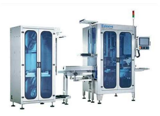
Labeling speed features ramp up and ramp down from 200BPM to 600BPM that effectively solve the problem of the first bottle falling down which easily occurs when high-speed starting.
