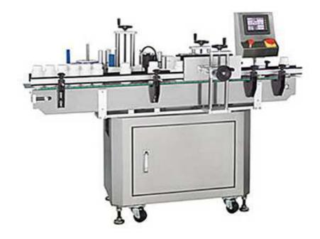
Model SLM-50 R, Suitable to apply accurate Labels on Double Side (Front & Back) of Flat/Oval/Square shaped products having PET, Plastic, HDPE, LDPE, Glass or any other surface.
