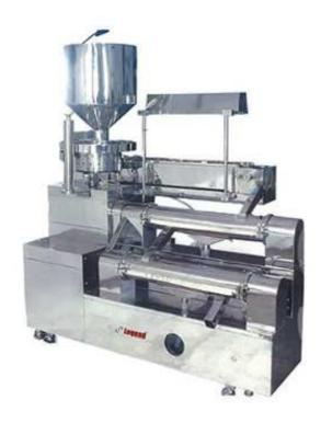
Legend Capsule Polishing Machine is a versatile machine used for polishing of capsules after filling operation. The capsules, while moving on the conveyor revolve along their axis due to the angular guides and thus can be inspected minutely. These machines are fitted with rotary spiral double brush Ultra polishing system that ensures a high gloss finish on the capsule.
