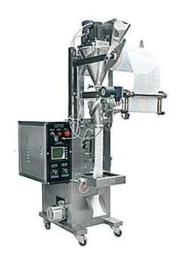
The machine is designed and manufactured specially for powdery and super fine powdery products. Driven by servomotor, the auger is rotating to fill products; furthermore, the filling range can be adjusted automatically through computer The processes of bag making, measuring, filling, sealing, cutting, counting and hot pressing codes can be done automatically. Packing material include several kinds of heat-seal lamination, such as PET/AL/PE, PET/PE, NYLON etc.
