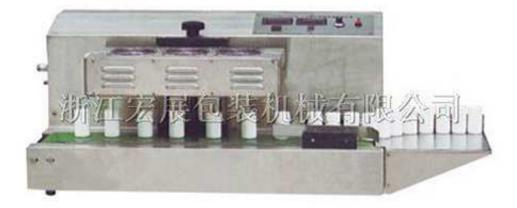
This series Portable induction sealing machine continuous induction sealing machine utilizes electrical magnetic induction principle to produce instant high heat to melt aluminum foil that hen adheres to the bunghole, reaching the aim of wet-proof, eakage-proof, mildew-proof and extending preservation time now it is widely used as sealing package machine in industries such as medicine, pesticides, lubricant and cosmetics etc.
