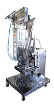
The MK-202 is semi pneumatic vertical forms fill seal packaging (VFFS) machine designed to package various free and semi free flowing liquid products. This machine uses volumetric piston dosing system to produce center sealed and 3 side sealed pouches / bags.
