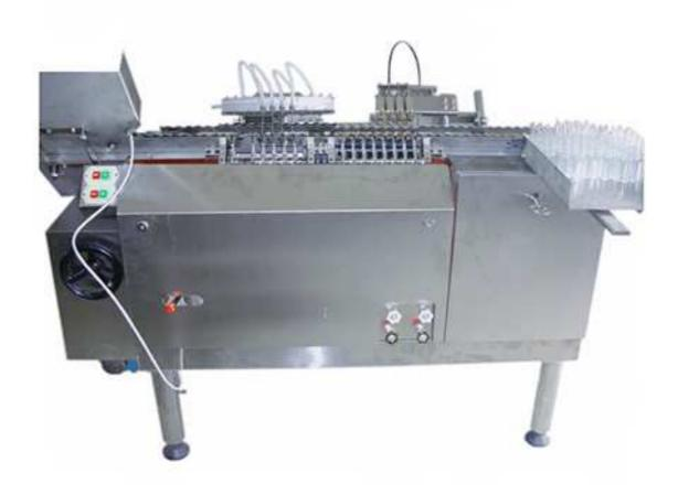
Filling and sealing machine for ampoule Model SLAG-4A is equipment specifilized in filling and sealing 1ml to 2ml, 5ml to10ml, and 15-20ml bottle in pharmaceutical works. This machine is equipped with automatic stop-filling device which can make filling case when there is no ampoule into filling station.
