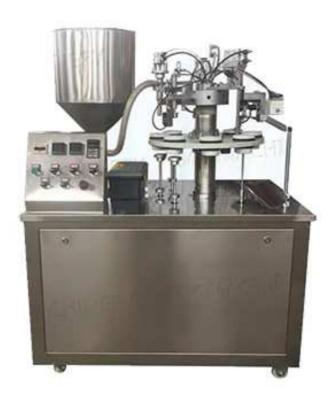
This machine is mainly used for plastic tube filling and sealing. It has been widely used in the fields of pharmacy, cosmetic, food and chemical etc.
