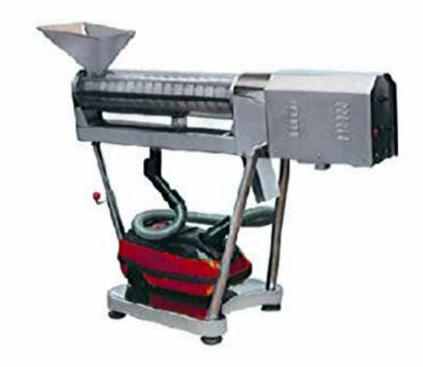
This polishing Equipment is a new pharmaceutical special equipment using in production of capsule and tablet. It is used to polish and clean dust and powder on the pills or capsules to get good smooth finish and can be up to hygiene standard of pharmacy industry.
