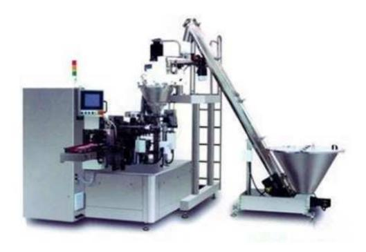
Granule Packing Machine is suitable for pharmacy, food, household chemicals, plastic products and other special industry and other loose type and in viscid granule material. Such as seeds, Chinese Drugs, feeding stuff, medicinal granules, pillar, monosodium glutamate, salt, sugar, soup blend, oat, tea, active carbon, washing powder, dryer, etc.
