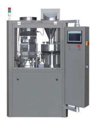
SED-2000J automatic capsule filler processes the products for optimal productivity up to 200000 capsules per hour, featuring low-maintenance operation, minimal downtime, and overall dependable production. Powder dosing uses the 5 stage tamping technology for an enhanced accuracy. Filling of pellets is available.
