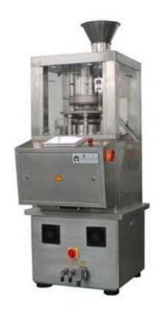
The machine is a single press automatic rotation for shape-pressing equipment, which have the function of press the grains material to be round or irregular shape tablets, such as candy, calcium tablets double-sides with letter printing and etc. which widely suitable for the Industries of pharmaceutical, Chemical, Foodstuff, Plastic Electronic, Powder Metallurgy and so on.
