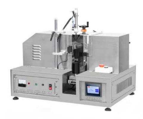
Packry's HX-007 ultrasonic tube sealing system that utilizes ultrasonic energy to produce a hermetic seal on most plastic and laminate tubes. It is ideal for lab use and low volume production jobs. The sealing capacity can reach at speeds up to 15 tubes per minute with diameters / cross-sections of tubes up to 50 mm.
