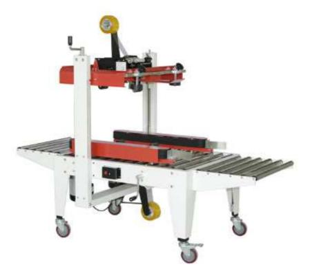
This machine's quality is better than so many carton sealing machines in Turkey. It is designed for saving time, and working with less worker. This machine automatically seal the top and bottom of the carton. And also it has belt which works with two motors, in top and bottom for taking the carton. It works best with 20-30 kg.
