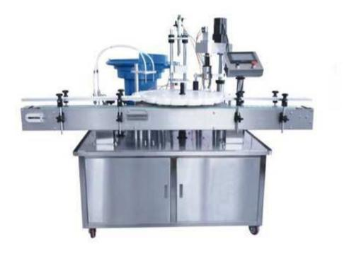
The machine is mainly applied to 50ml or less electronic cigarette oil, eye drops, nail polish, eye shadow, essential oils and other products of automatic filling, plug and screw cap.
