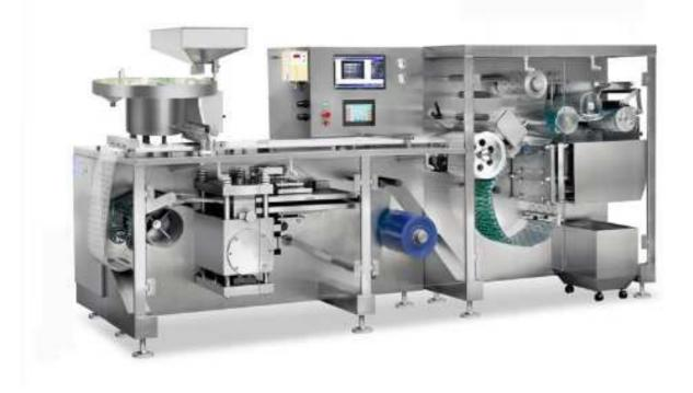
This series machine is at high precise and the latest roller and plate type blister packing machine, developed by our company. It applies to pharmaceutical industry, food industry, medical appliance and electronical area. It is suitable for packing capsules, tablets, milk pieces, candy, electronical element and similar material, with sealing packing in al-pvc, paper-pvc
