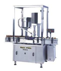
Pack Well Automatic Screw Capping Machine is versatile, self-supported on stainless steel leg with height adjustable adjustment system. The machine is precision built on sturdy welded steel frame completely enclose in stainless steel sheet and doors are providing to facilitate the servicing of machine.
