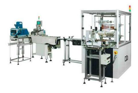
The semi-auto model OSA-380 is good for hard square box. It adopts either shrinkable or non-shrinkable BOPP film to be folded on sides of box. It can have perfect packaging work without wasting trimming. Because of cheap price, it can save packaging cost & reduce labor cost. This machine is controlled by HMI, which is more human friendly without strict limitation by package sizes. The Auto Collator is an option to pack multiple products without needing box for cost saving.
