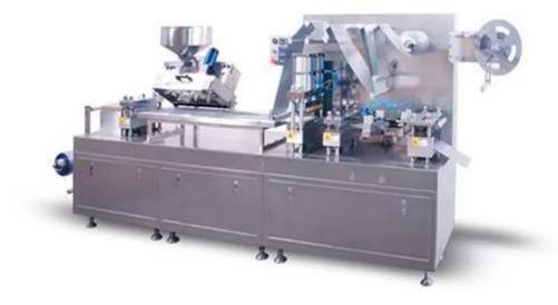
This machine is designed and improved by our technician according to the feedback of our customers who have been using our products for many years. It is widely used in the of medicine, food, electron, hardware for Alu/PVC blister packing of various nubby object and liquid. It has effect of moisture proof and dust-proof, and enhancing level and additional value of products. It can also be linked to work with pillow-type packing machine and boxing machine.
