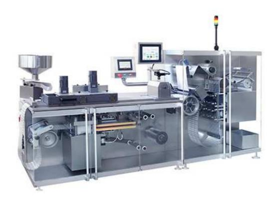
This machine is suitable for automatic high speed alu pvc packing of capsules, tablets and chewing gums, candies. It adopts flat pressure forming to form strong and average blisters, and roller type mesh sealing to ensure reliable sealing. The machine is equipped with batching system, embossing device and horizontal boundless punching to achieve high production capacity and greatly save packing material.
